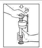
Replace TOP by engaging lugs and rotating 1/8 turn clockwise. MAKE CERTAIN TIP IS TURNED TO THE LOCKED POSITION. VALVE MAY NOT TURN ON IF TOP IS NOT FULLY TURNED TO THE LOCKED POSITION.
